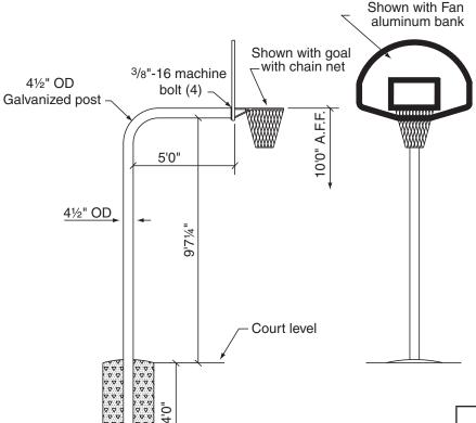
Specifications-EZ Fold 5064XY **Outdoor Backstop** 41/2" Gooseneck Post with 5' Extension
